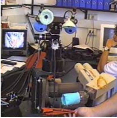
Figure 1 – The experimental setup. The 12 degrees of freedom humanoid robot described in the experiment.
