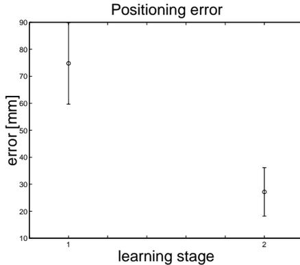
Fig. 11. Endpoint positioning error before and after learning. The error expresses the Euclidean distance between the end effector and the target at the end of reach. 134 movements were executed during the learning phase. The maximal achievable precision of the arm was 30mm.
