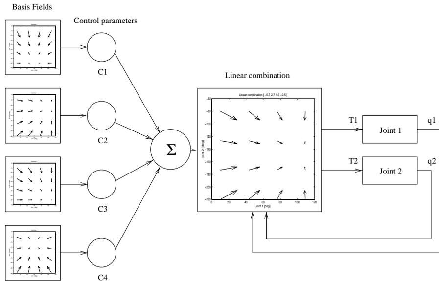
Fig. 1. Controller structure: motor primitives, represented by torque fields are combined (weighted by  $C_1$ ,  $C_2$ ,  $C_3$  and  $C_4$ ). The overall field “guides” the arm end-point toward its EP.
