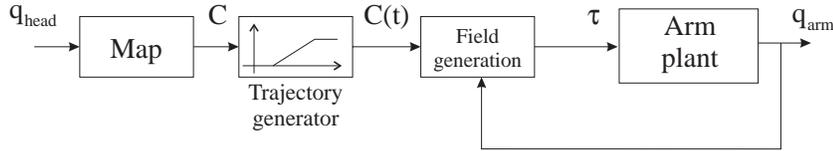
Fig. 9. The overall arm’s control scheme. The position of the head ( $q_{head}$ ) addresses the map which outputs the activation vector for the arm. This stage is followed by a trajectory generation which interpolates linearly between activation vectors. The resulting force field is then computed and used to generate the torques which drive the arm motors.
