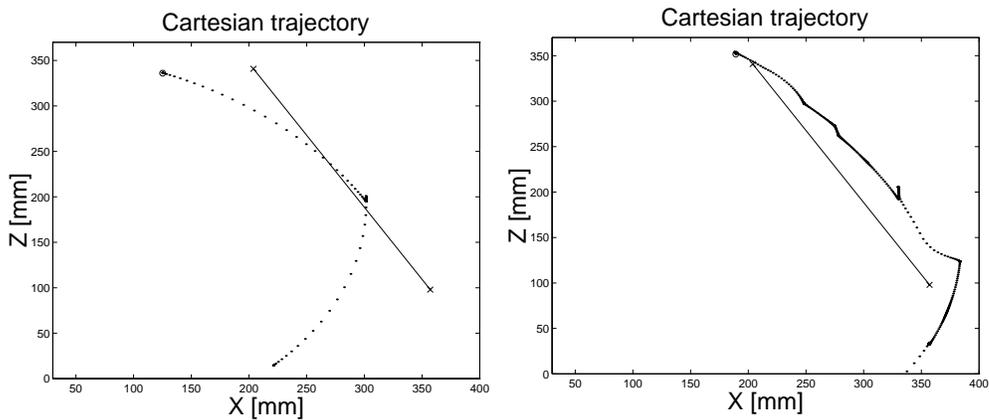
Fig. 14. Tracking a moving target. Abscissa and ordinate are the  $X$  and  $Z$  position represented respect to the arm base frame. The target moves in both experiments from the lower-right to the upper-left position at constant velocity along a straight path (solid line). The dotted line represents the end-point trajectory. The left plot has been obtained using the map before training, the right one refers to the map after training.
