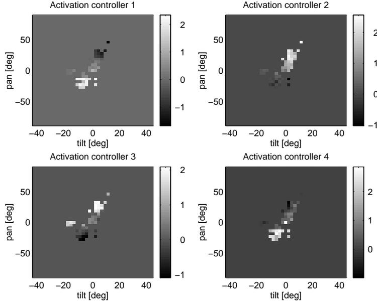
Fig. 10. Head-arm mapping after training. Ordinate and abscissa are the head joint angles (in degrees). Grey levels represent activation value  $C_1$ ,  $C_2$ ,  $C_3$  and  $C_4$  of each controller (see section 2.1).
