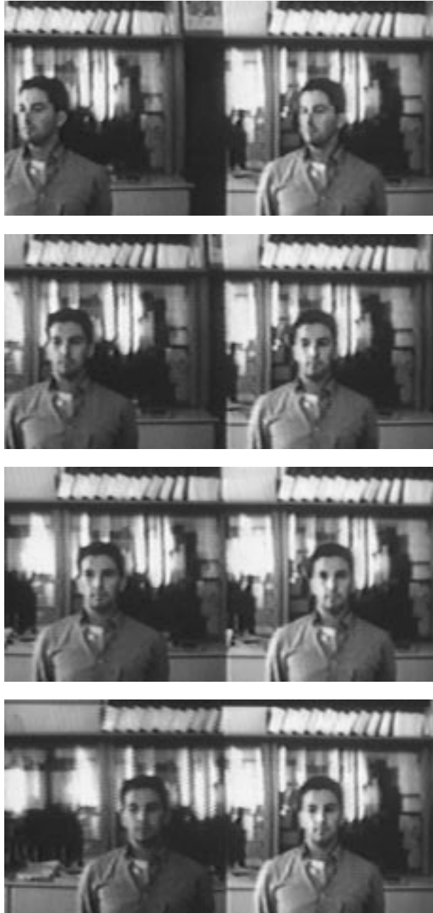
Figure 13: Binocular frames during stabilization experiment. Left: non stabilized camera; right: stabilized camera.
