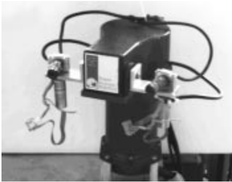
Fig. 3. The head mount. Left: front view of the robot head shows the offset position of the cameras with respect to the neck rotational axis (head geometrical parameters, \mathbf{b}= 136 mm, \mathbf{a}= 95 mm). Right: the artificial "vestibular" system is rigidly fixed on the back of the head mount.
