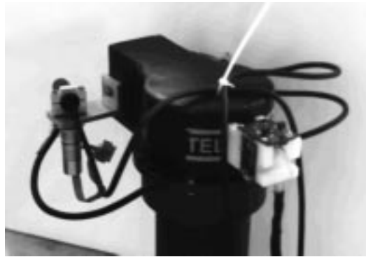
Fig. 3. The head mount. Left: front view of the robot head shows the offset position of the cameras with respect to the neck rotational axis (head geometrical parameters, \mathbf{b}= 136 mm, \mathbf{a}= 95 mm). Right: the artificial "vestibular" system is rigidly fixed on the back of the head mount.
