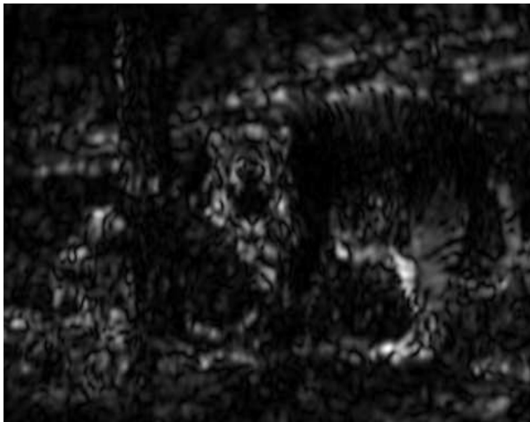
Figure 2.2: Complex cells output to the image in figure 2.1 for 0 degrees filter of formula (2.1).
