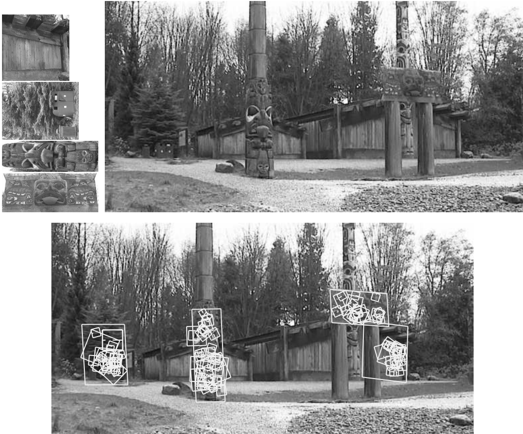
Figure 13: This example shows location recognition within a complex scene. The training images for locations are shown at the upper left and the 640x315 pixel test image taken from a different viewpoint is on the upper right. The recognized regions are shown on the lower image, with keypoints shown as squares and an outer parallelogram showing the boundaries of the training images under the affine transform used for recognition.
